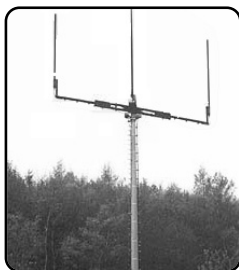
Omnidirectional base station with a single cell
