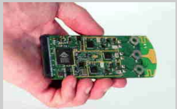
Airgo Networks' MIMO PC Card. Note multiple antennas on right. Source: Airgo Networks
