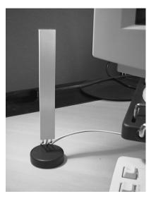
Use the Range Extender Antenna when the integrated antennas of the PC Card are concealed or shielded, for example:
